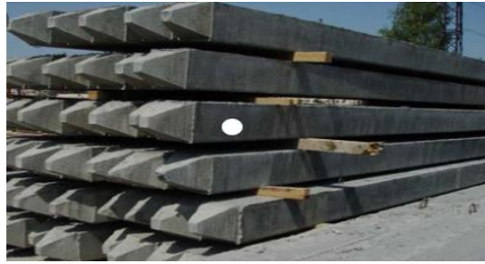
Gambar 3. 2 Tiang pancang beton precast reinforced concrete pile
